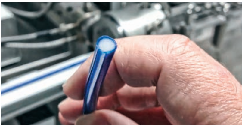
Co-extrudate of API core with Soluplus® Pharma Polymer (BASF) outer layer formed using a hot melt extrusion process with Pharma 16 and Pharma 11 Twin-Screw Extruders.
