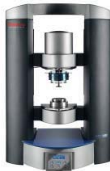
Рис. 1. HAAKE MARS (Modular Advanced Rheometer System) III
